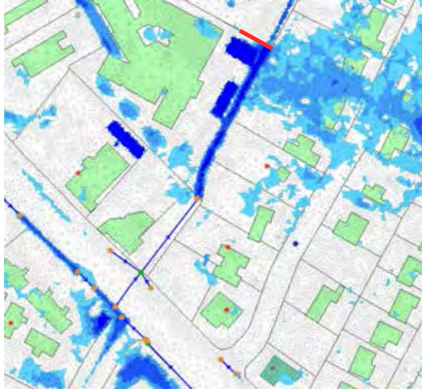
Figure 8: 100-yr with Channel Blockage at Fence
