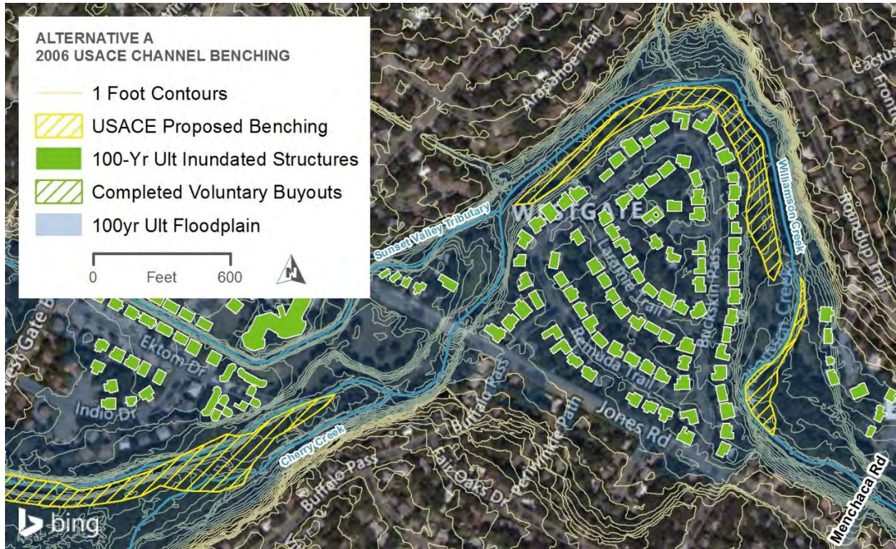
Figure 5-3. 2006 USACE Recommended Channel Benching at Broken Bow
