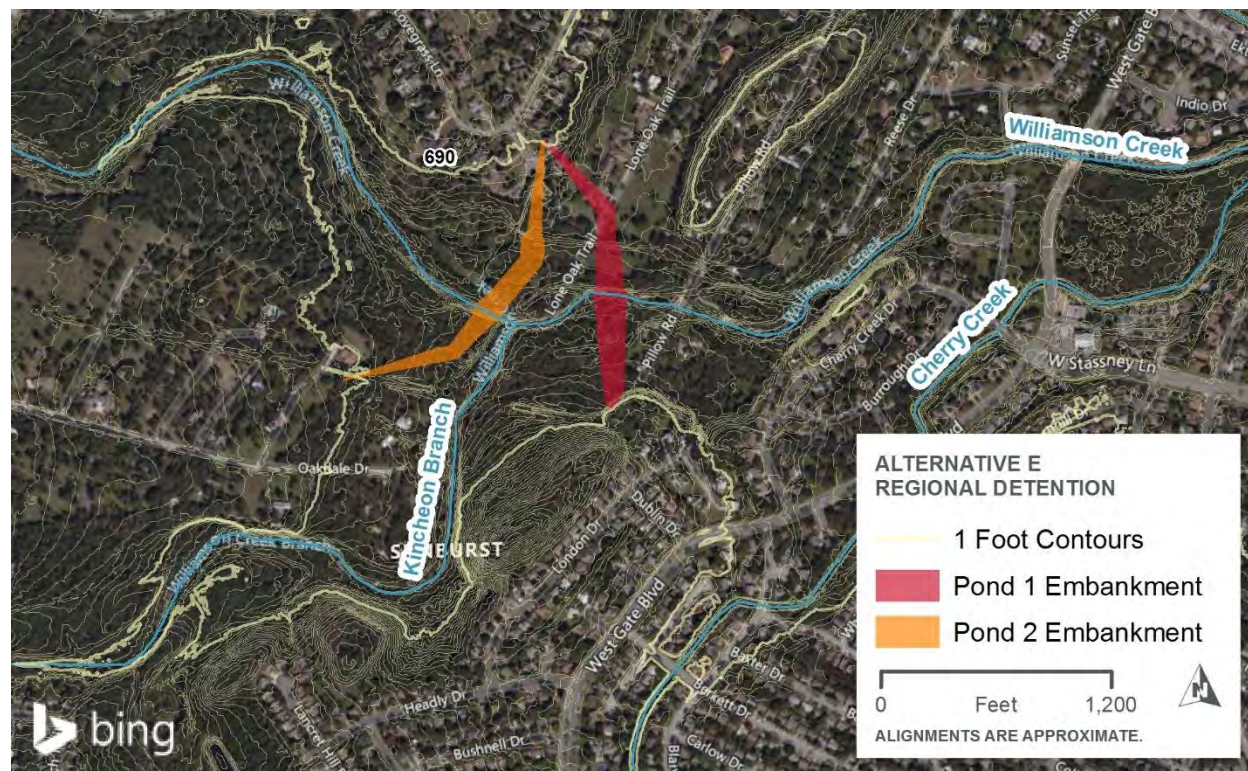
Figure 5-14. Alternative E – Regional Detention Conceptual Layout
