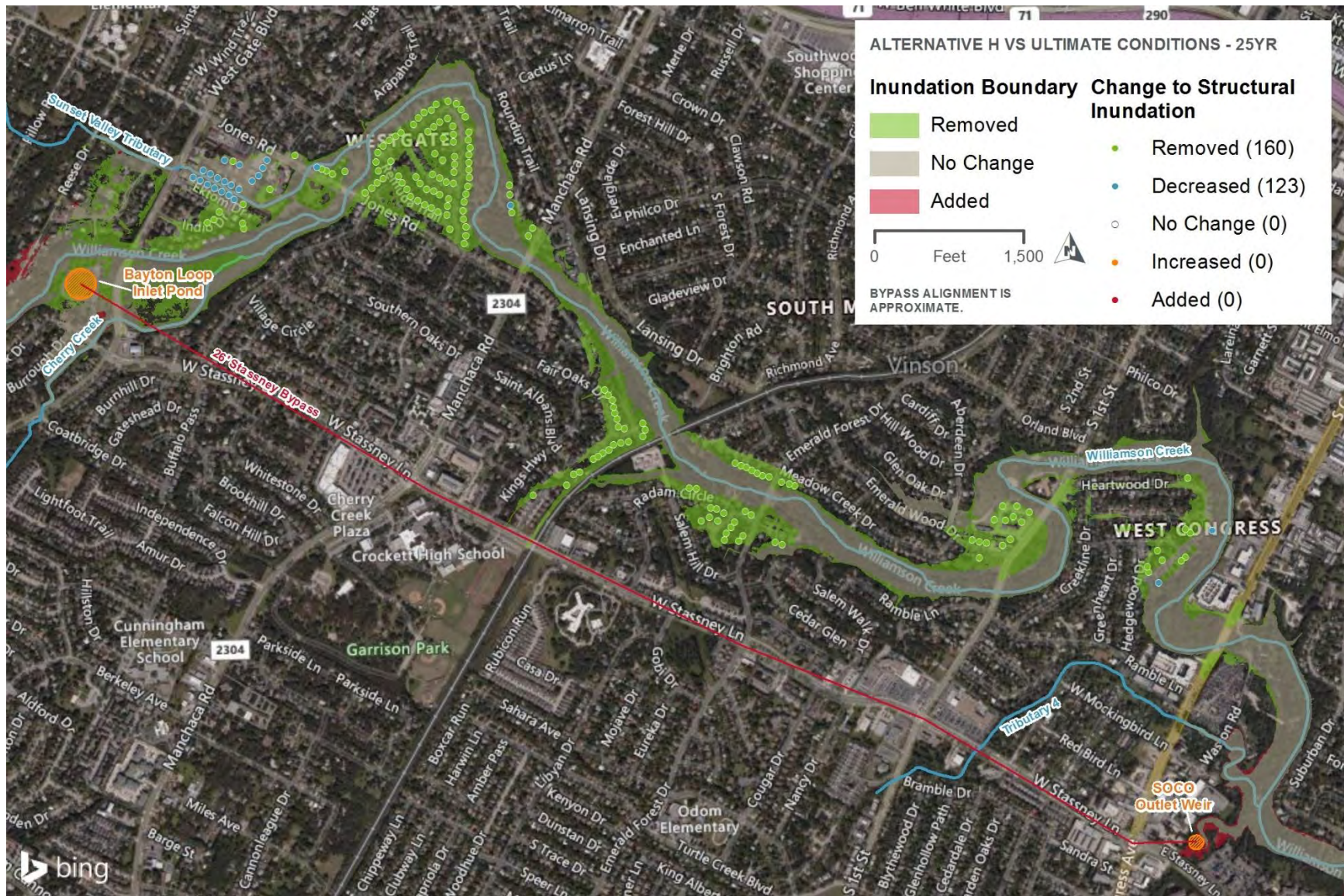
Figure 5-44. Alternative H vs Ultimate Conditions – 25yr: Change to Structural Inundation
