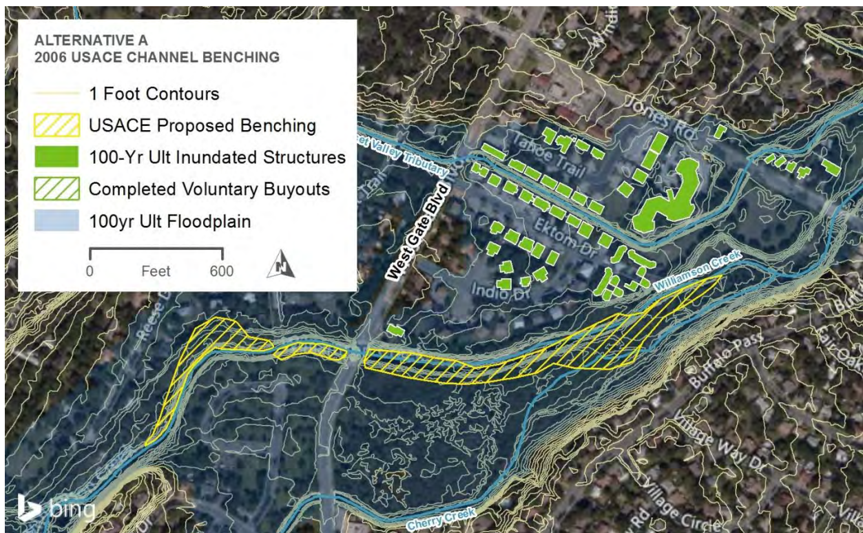
Figure 5-4. 2006 Recommended Channel Benching at Westgate/Bayton Loop
